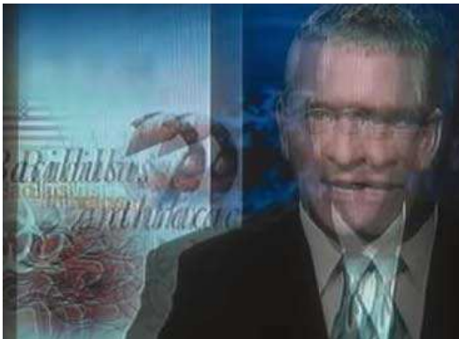
Fig. G. Ghosting (on a colour LCD)
