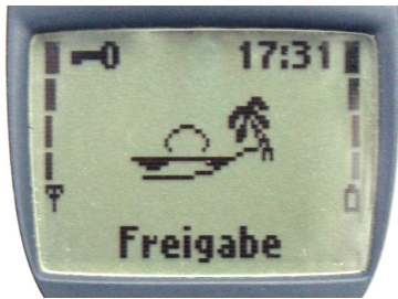
Fig. E. Monochrome graphic displayed on the liquid crystal display of a Nokia 3310. This display is in the form of a grid, 84 pixels wide and 48 tall.
