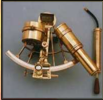
Sextant: Spinning mirror on gyroscope
