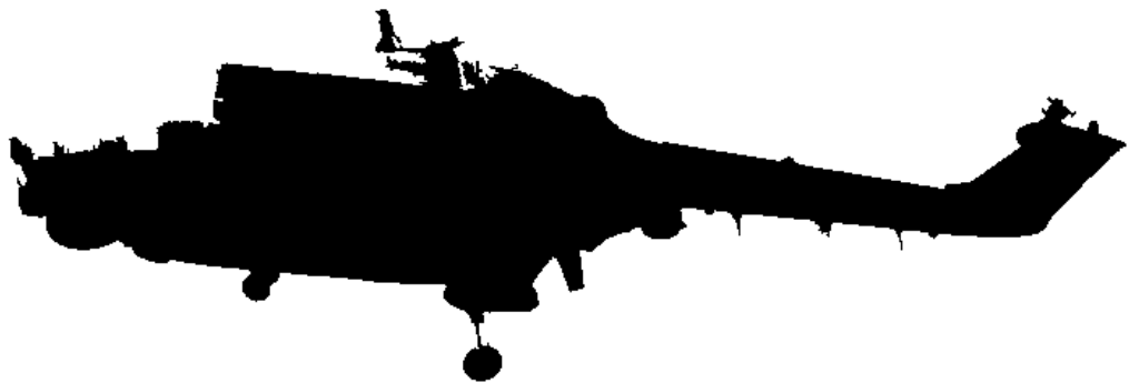
Figure 3-1: The Threshold-filtered image has been grouped by a Hoshen-Kopelman algorithm, and small groups have been removed from the image.
